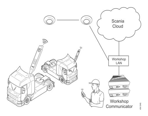
When the vehicle arrives, the user places a VCI in the vehicle and turns the key to drive mode. SWS automatically reads all relevant information from the vehicle, checks for which control units new software is available and presents the vehicle in the cloud service.
