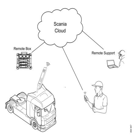
When troubleshooting vehicles in the workshop, the mechanic connects VCI to the vehicle. The key is set to drive mode. In SWS, the user starts the job and establishes a connection by selecting the vehicle, which is displayed by its chassis serial number. Depending on the type of fault the mechanic is looking for, they use fault codes, wizards or checks etc. to be able to call in the fault.
